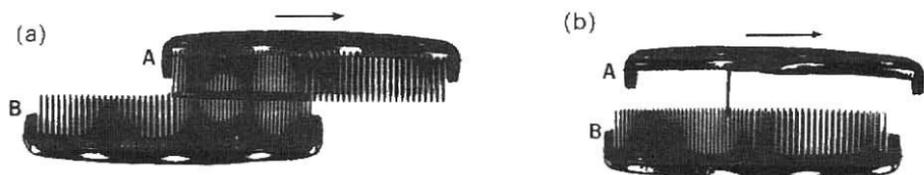
**Fig. 11.1.** Haircomb models illustrating the origin of atomic-scale friction. (a) Sliding friction at an “ideal” A–B interface. (b) Sliding friction as observed in a friction force microscope (a modified SFM capable of measuring forces in the direction of the trajectory). The teeth of the combs represent atoms at the surface of materials A and B
