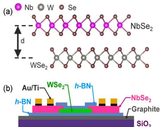
FIG.1.  $\text{WSe}_2$  field-effect transistor with conducting  $\text{NbSe}_2$  leads in side view. Atomic-model representation of the  $\text{NbSe}_2/\text{WSe}_2$  interface (top) and schematic structure of the device (bottom). (From Ref. [2]).
